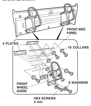
9. Reinstall the front bed panel and the upper tiedown hooks.
