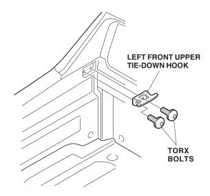
2. Remove the front bed panel (six torx bolts).
